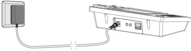
Figure 26 Schematic Diagram of the NPM Power Supply Cable Connection
